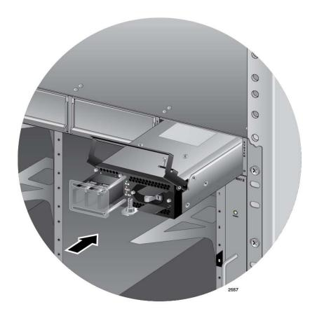
Figure 67. Inserting the AT-SBxPWRSYS1 DC Power Supply
